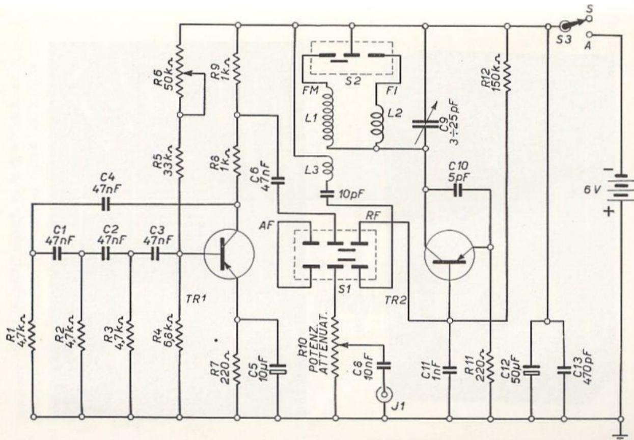
Fig. 12.16 - Generatore FM a transistor.
