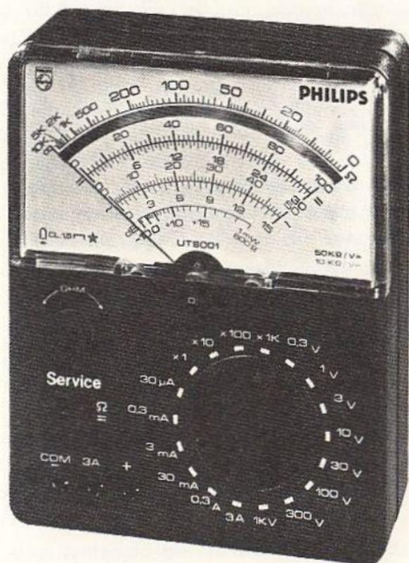
Fig. 6.6 - Multitester Philips mod. UTS-001.
